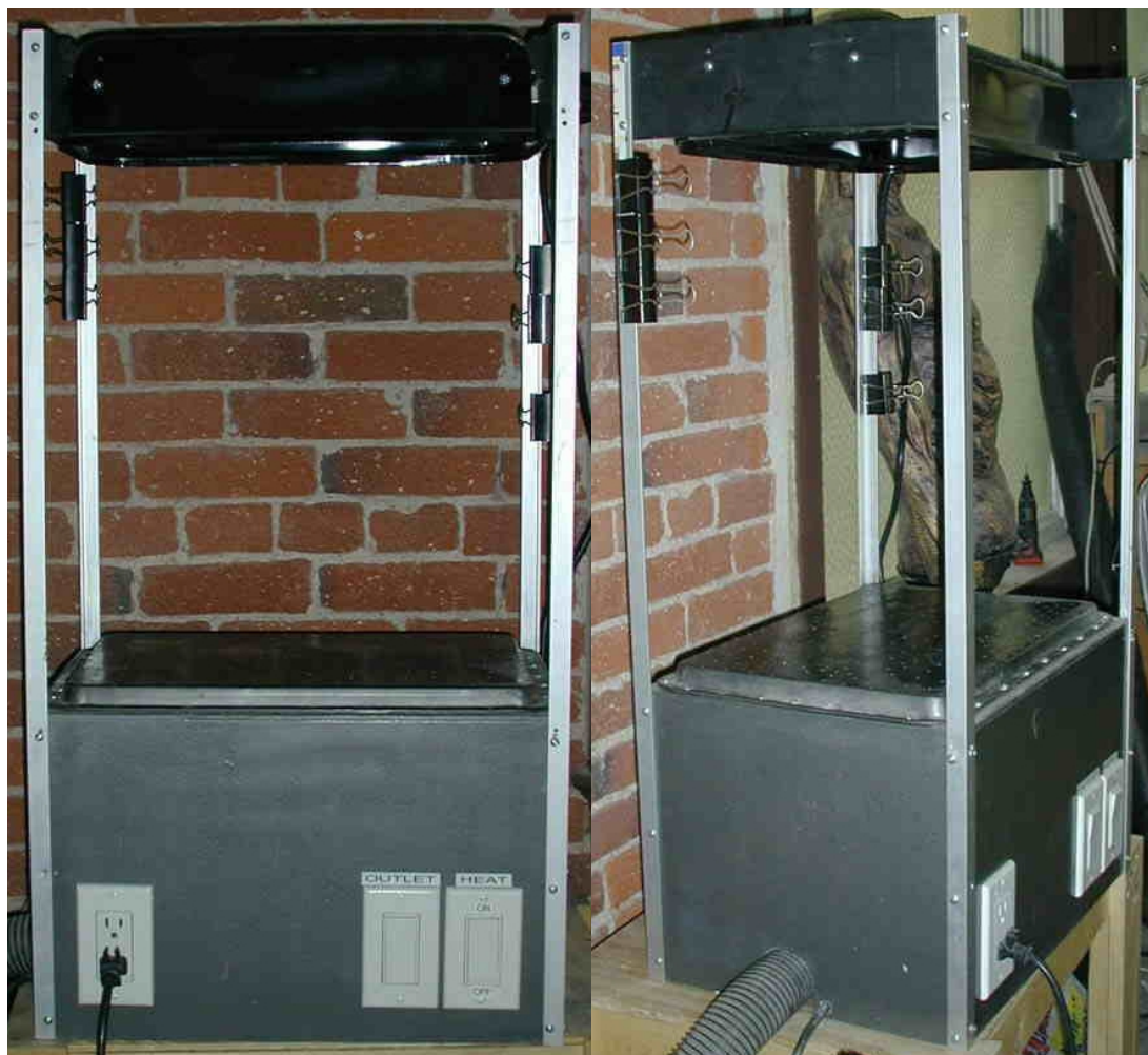
Front and side view of vacuum forming table made by "Ralis Kahn". (Note the corpse on the right side of the vacuum forming table....very nice touch!)
